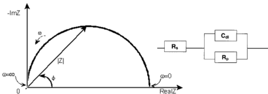
Figure 1: Nyquist plot of the Randles circuit (left) and the Randles circuit (right).
